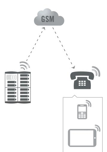
The **myCom** entry system comprises of just a GSM module, power supply and the option of keypad entry. All communications are made via the GSM technology, which is all housed in the front call station.
